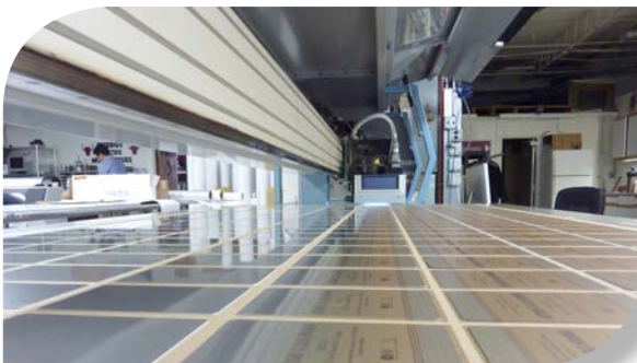
Second side is printed in precise registration
