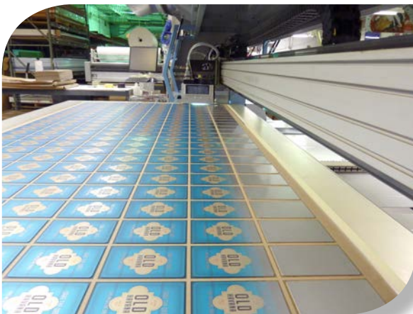
High-resolution UV printing on aluminum plates
