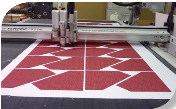
High-speed Zund G3 digital cutter with specialized rotary fabric cutting tool, cuts up to 10x faster than other blades and with cleaner edge
