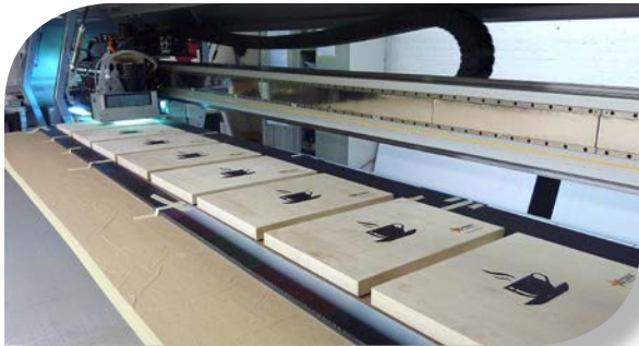
Wood box lids being printed on our UV flatbed press
