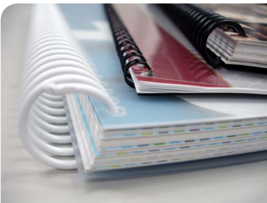
Double-O wire and spiral coil binding
