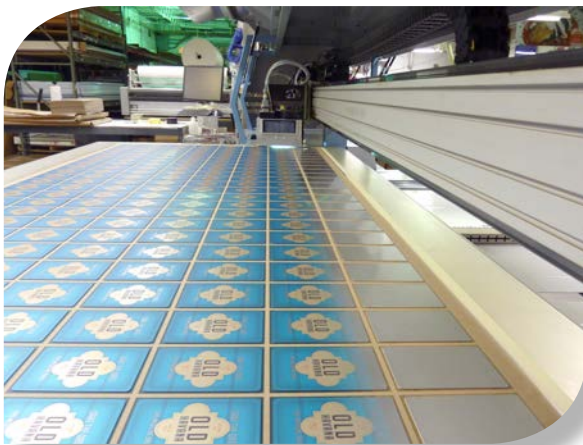
High-resolution UV printing on aluminum plates
