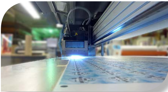
UV lamp cures ink instantly with excellent scuff resistance and durability
