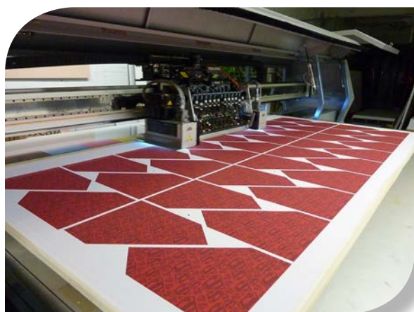
Magnetic Linear Transport on UV flatbed printer produces banding-free output
