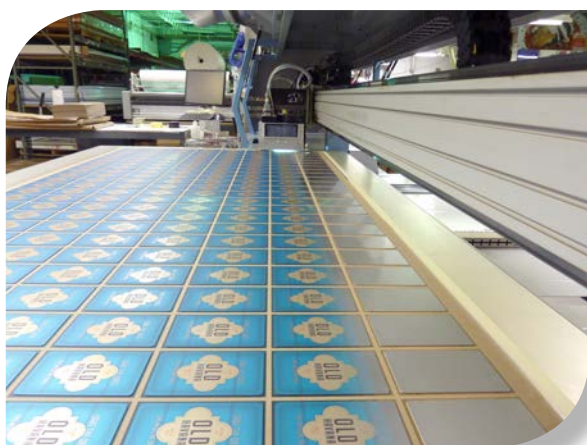
High-resolution UV printing on aluminum plates
