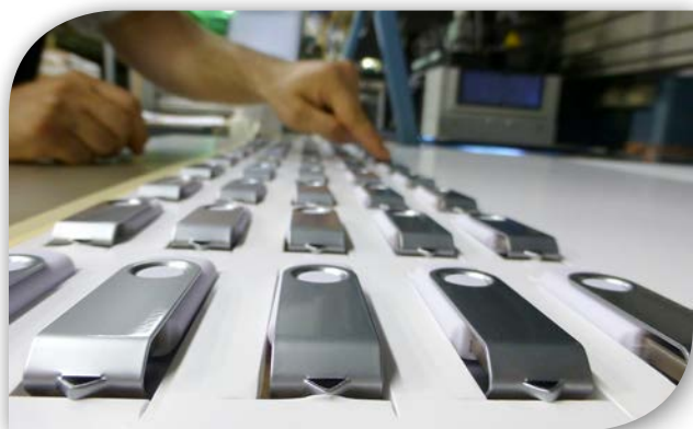
Custom templates ensure accurate positioning
