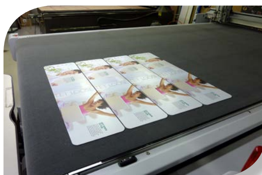
Panels being cut on CNC digital router
